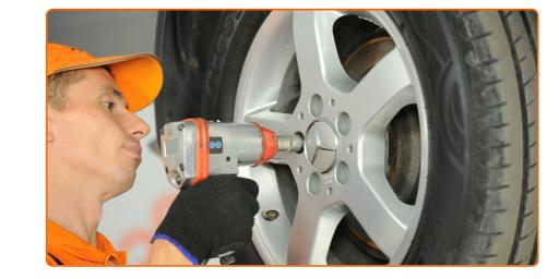
Screw in the wheel bolts. Use wheel impact socket #17.
