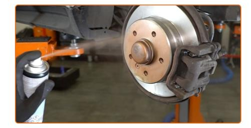
Treat the surface where the brake disc contacts the wheel rim. Use copper grease.
