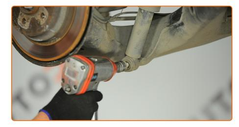
Unscrew the lower fastener of the shock absorber. Use a drive socket #21. Use a ratchet wrench.
