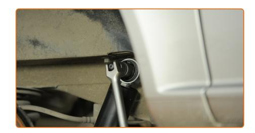
Tighten the top shock absorber fastening. Use a drive socket #21. Use a torque wrench. Tighten it to 87 Nm torque.
