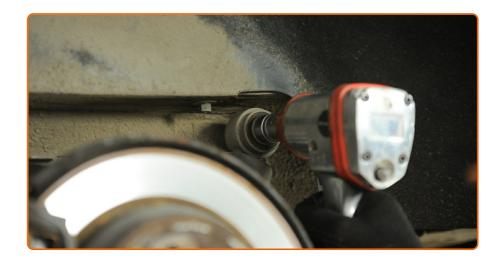
Unscrew the upper fastener of the shock absorber. Use a drive socket #21. Use a ratchet wrench.
