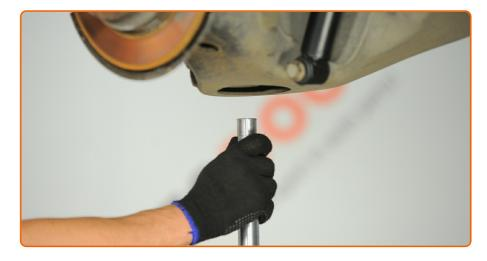
Remove the support from under the arm.
