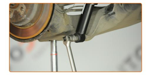
Tighten the lower fastener of the shock absorber. Use a drive socket #21. Use a torque wrench. Tighten it to 87 Nm torque.
